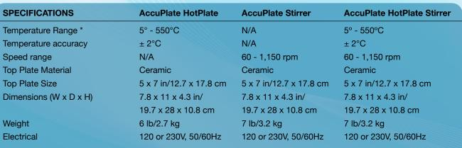
\*Temp range when using external temp controller is 5-200° C
